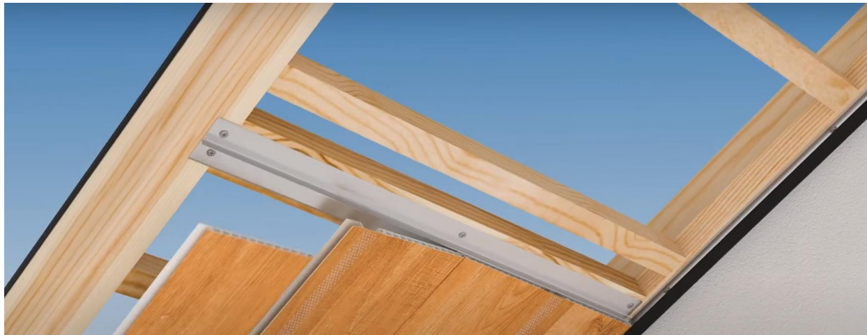
Figure 11, Details at soffit, H-Mold Trim
