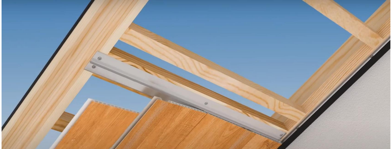
Figure 11, Details at soffit, H-Mold Trim
