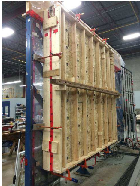
Figure 3: Wall construction showing horizontal brace at mid-height.
